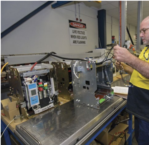
NHP's Air Circuit Breaker manufacturing facility, Laverton Victoria.
